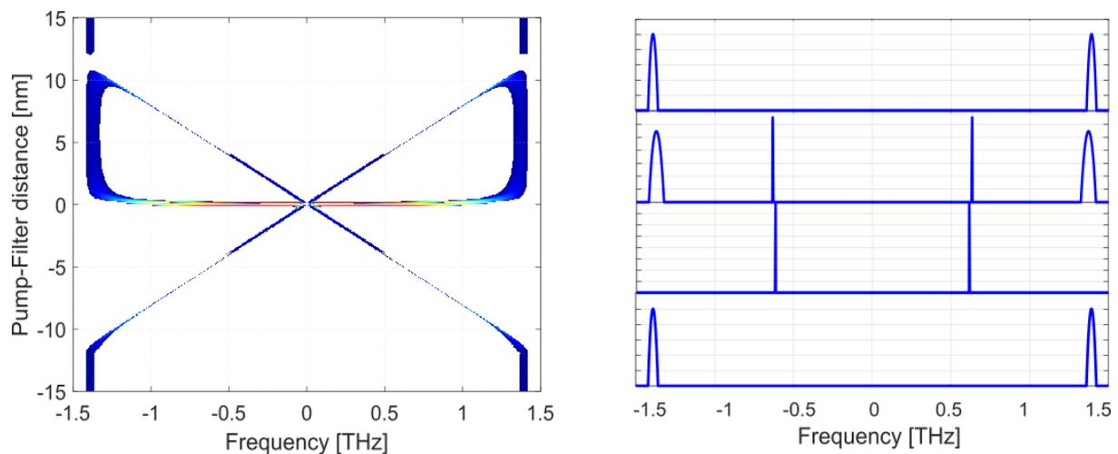
Figure 3: Evolution of the parametric gain as function of pump-filter distance
