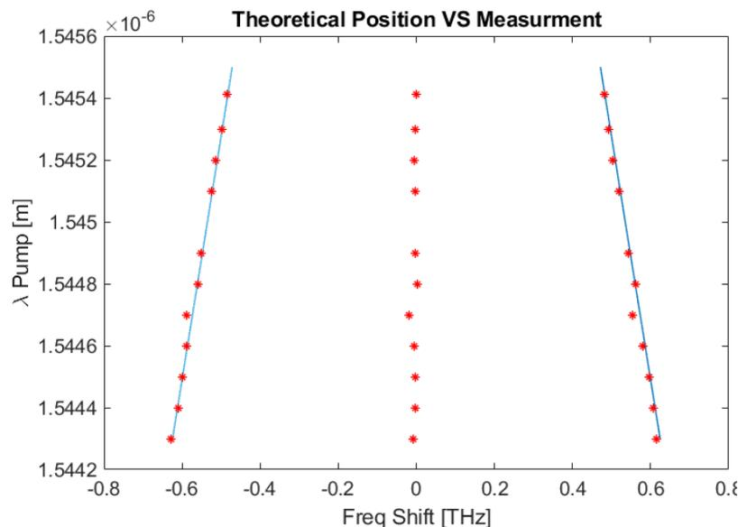
Figure 2: Demonstration of the tunable capability of the GTF process, with the pump positioned at 1545 nm.
