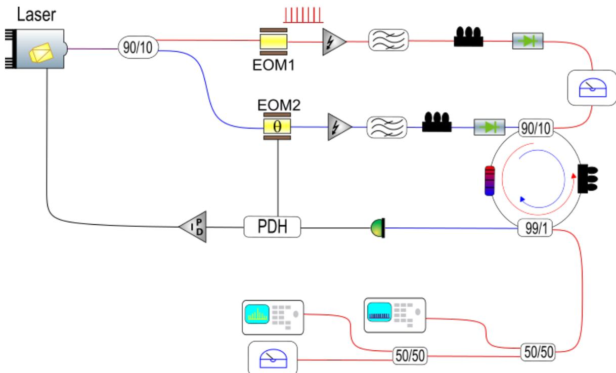
Figure 1: Experimental setup realized for the main characterization of GTF process in a fiber cavity. All the main elements of the setup are not polarization maintaining.
